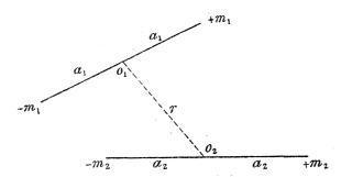
The mutual potential energy of two such bar-magnets is easily worked out as follows.
